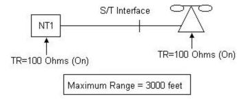
Fig. 5: Terminating Resistor Range
